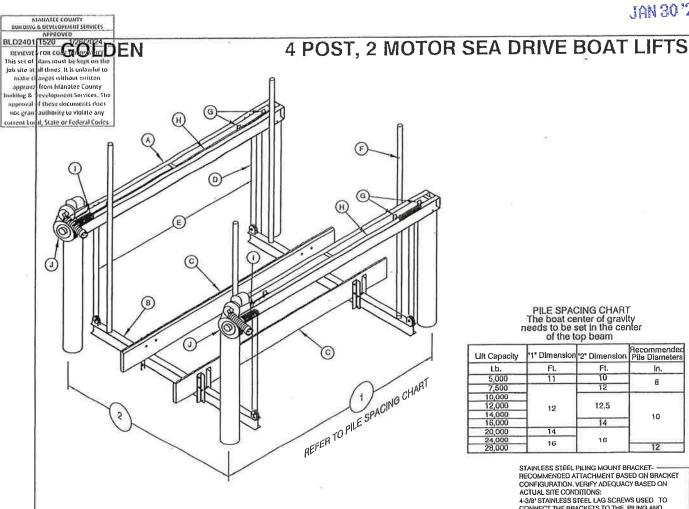
PILE SPACING CHART The boat center of gravity needs to be set in the center of the top beam
